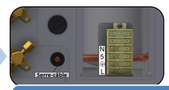
Step 2: Connect the connections housing and the outdoor unit through the cable tie with the 4G1.5 cord (not supplied) as shown in the wiring diagram (see section 3.6.4, p 20).
